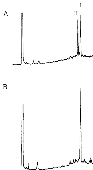
Figure 2. (A) Reverse-phase HPLC of I, synthesized by standard methodology, revealing major byproduct II. (B) Treatment of the above mixture with hydrazine converted II to I; Vydac C 4 , 5 μm, 20% B to 35% A over 30 min. A = 5% CH 3 CN containing 0.1% TFA; B = 0.1% TFA in CH 3 CN.
